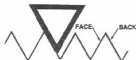
HANDSAW IS CROWDED TO THE RIGHT SO THE FILE IS HEAVY AGAINST THE BACK OF THE TOOTH (THIS IS ACCOMPLISHED BY INCREASING THE RED FEED STROKE KNOB)
