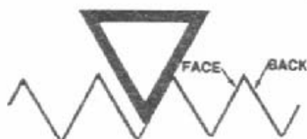
HANDSAW IS CROWDED TO THE LEFT SO THE FILE IS HEAVY AGAINST THE FACE OF THE TOOTH (THIS IS ACCOMPLISHED BY DECREASING THE RED FEED STROKE KNOB)
